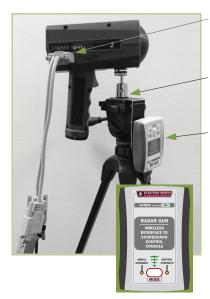
**Serial Data Port** = Connects the Radar Gun to the Interface, faciliating wireless data transmission to the Control Console. Simultaneously allows the Gun to receive power from a Battery Pack using a Y-Cable, in lieu of 6 AA batteries.
