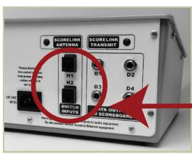
serves only to connect the wired Switch Assembly to your Control Console.
