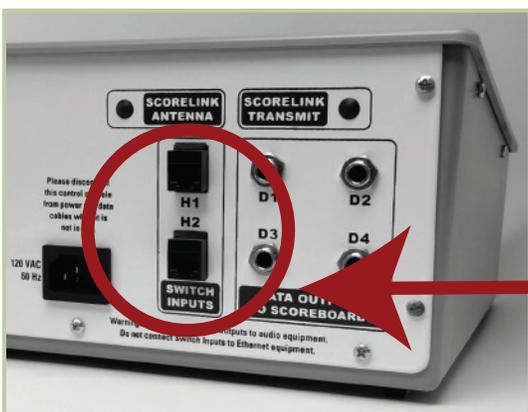
Connect the Switch Assembly to the back of the Control Console using either of the "H" labeled **Switch Inputs**. Note: Older back plates specify a particular handheld unit for each input. However, these older inputs are also interchangeable.
