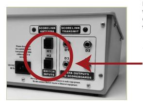
cord serves only to connect a wired Switch Assembly to your Control Console. Do not attempt to connect either the Switch Assembly or the Control Console to a network or PC using this cord or the RJ-45 sockets.
