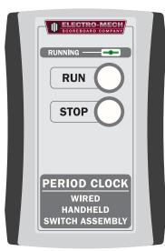
Running Indicator Light = Illuminates solid green when the Period Clock is running. Note: this LED may not function consistently when the device is attached to an older Control Console.
