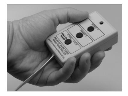
If you purchased a set of Play Clocks (also called Delay of Game Timers or 25-Second Clocks), your package includes a handheld three-button controller. This controller plugs into the back of the control console using the RJ-45 style connector at the end of the handheld unit's cable. You may plug into either of the two console sockets labeled "SWITCH INPUTS" on current models, or either the "CLOCK Hand-held" or "DGT/SC Hand-held" socket on older models. Here's what the buttons do:
