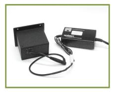
**Charging:** Remove the B10 Battery Pack from the control console and connect it to the Universal Smart Charger, using the barrel-style adapter. The LED indicator on the charger will glow red during the charge cycle and turn green when charging is complete. Typical charge time is a mere two hours.
