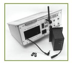
**Applying Power:** Set the three-position power switch on the back of the control console to the top "BATTERY POWER" position. On a fresh charge, the B10 Battery Pack will run an MP console with embedded ScoreLink system for over 12 hours.
