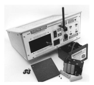
• Remove the battery holder and take out the ten nickel-metal hydride (NiMH) battery cells.
