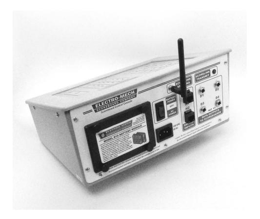
When you are ready to use the control console, click the power switch up into the "BATTERY POWER" position.
