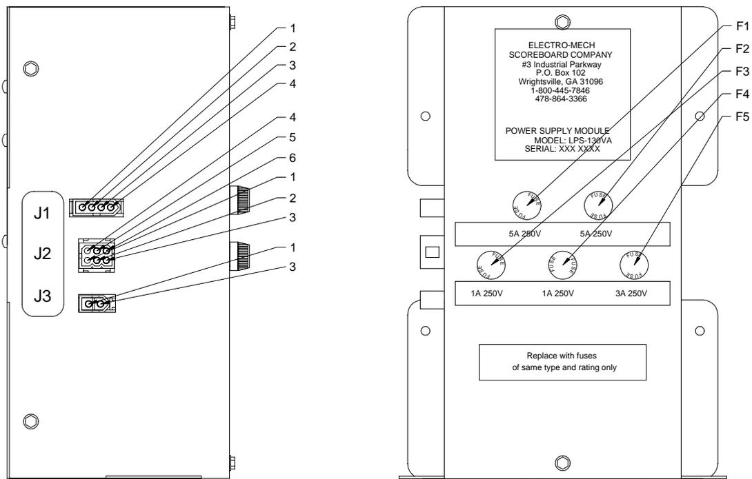
**Figure 9 LPS-130VA POWER SUPPLY MODULE**
