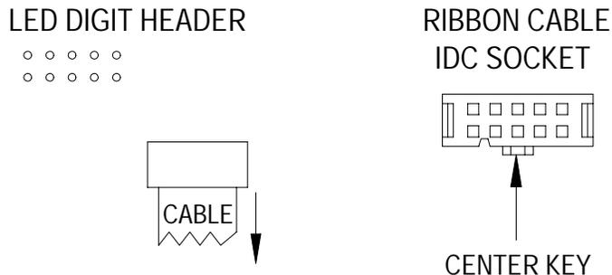
CENTER KEY ON RIBBON CABLE IDC SOCKET
