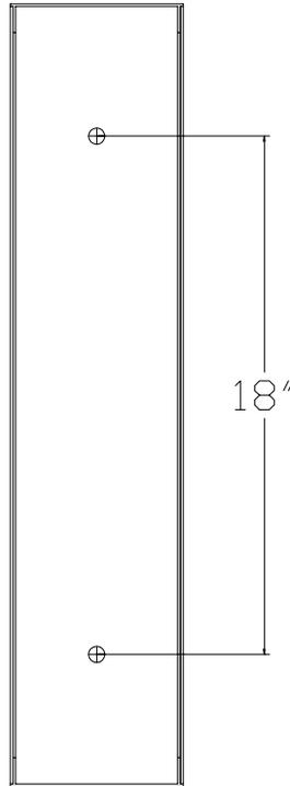
**Figure 1 Model 2150 Mounting Points**
