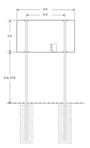
Once you have verified the positions of the posts and the size of the footings, you are ready to dig your holes, pour your concrete, and set your posts. There are several techniques for ensuring proper alignment of the posts. Typically installers will construct a temporary wooden support frame to hold each post in place while the concrete sets. Having plumb posts in the proper position is the key to a smooth mechanical installation.
