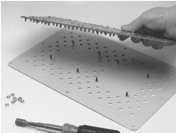
The LED circuit board is held to the mask by several nuts, which you can remove using a 3/8-inch nut driver. On outdoor displays the thick conformal coating can be messy, as the lock washers on the nuts dig into the coating and knock pieces of it away. Be careful to keep the whole assembly right side up when you return it to the practice segment timer cabinet.
