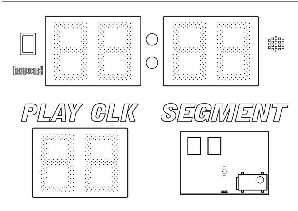
If your scoreboard system includes a ScoreLink wireless data kit, the receiver unit will be in the upper left corner of the display face, and the internal Horn will be mounted in the upper right.
