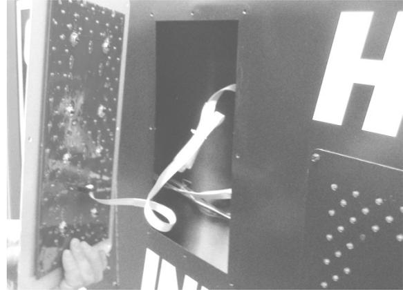
If your purpose in removing the LED assembly was to provide access to the components behind it, you may skip the next part about removing and replacing the LED printed circuit board.
