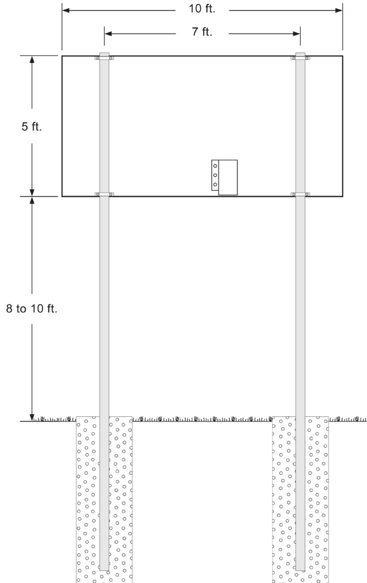
Once you have verified the positions of the posts and the size of the footings, you are ready to dig your holes, pour your concrete, and set your posts. There are several techniques for ensuring proper alignment of the posts. Typically installers will construct a temporary wooden support frame to hold each post in place while the concrete sets. Having plumb posts in the proper position is the key to a smooth mechanical installation.
