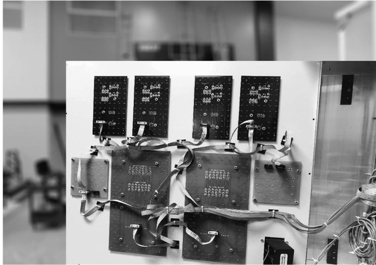
Each LED circuit board is held to the face by several nuts, which you can remove using a 3/8-inch nut driver. Be careful to keep the PCBs right side up when you return them to the shot clock cabinet.
