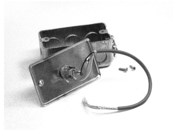
The splice point should stay inside the junction box. That is, you want to feed the long run of cable into the box rather than pulling the pigtail out. Electro-Mech provides a strain relief on one side of the junction box to secure the cable. You may choose to connect conduit directly to the junction box, in which case the strain relief will not be needed. The junction box is designed to accept 3/4-inch conduit fittings.
