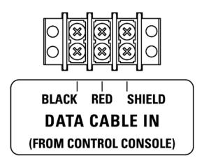
You may purchase data cable from the factory, or you may source it elsewhere. We recommend (and supply) cable that is rated for direct burial. It includes two insulated 22 AWG stranded conductors (red and black), along with a non-insulated conductor, all wrapped by a braided or foil shield. This document will discuss, in a few pages, what the other end of this cable is connected to.
