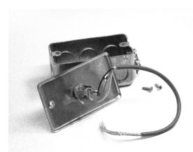
The splice point should stay inside of each junction box. That is, you want to feed the long run of cable into the box rather than
