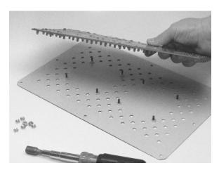
The LED display circuit board is held to the mask by several nuts, which you can remove using a 3/8-inch nut driver. On outdoor displays the thick conformal coating can be messy, as the lock washers on the nuts dig into the coating and knock pieces of it away. Be careful to keep the whole assembly right side up with you return it to the play clock cabinet.
