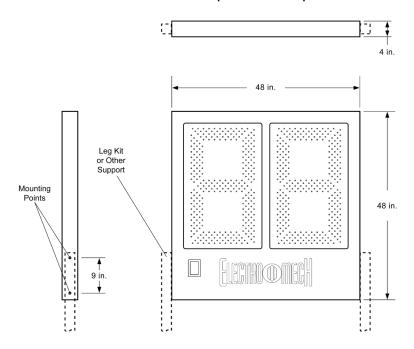
If you wish to attach your play clock displays to a different support structure, you may take advantage of the mounting plates included in the cabinets. These plates have tapped holes, spaced nine inches center-to-center, along the sides of each cabinet. The tapped holes accept 1/2-inch-13 threaded bolts. For Model LX3030, support brackets or posts would need to be positioned 48 inches apart (inside spacing) to provide room for the cabinet.
