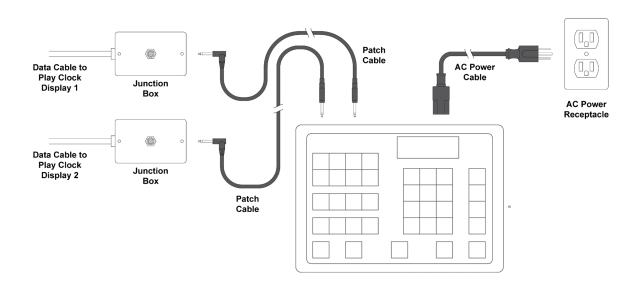
If your play clock package includes a ScoreLink RF Communications system, the power receptacle may be the only consideration on the control console side of the installation process. For details about ScoreLink, consult the documentation that ships with the product. Otherwise use the stereo patch cables to plug the console into the junction boxes.
