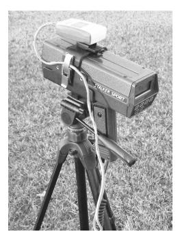
Your scoreboard package includes a radar gun kit. The radar gun can capture the speed of pitches and relay that information to your control console, which sends the data to be displayed on your scoreboard. The radar gun is battery operated and therefore does not require AC power during the game (as long as you keep the battery charged). It communicates wireless with the scoreboard control console, so there are no additional cables to run.
