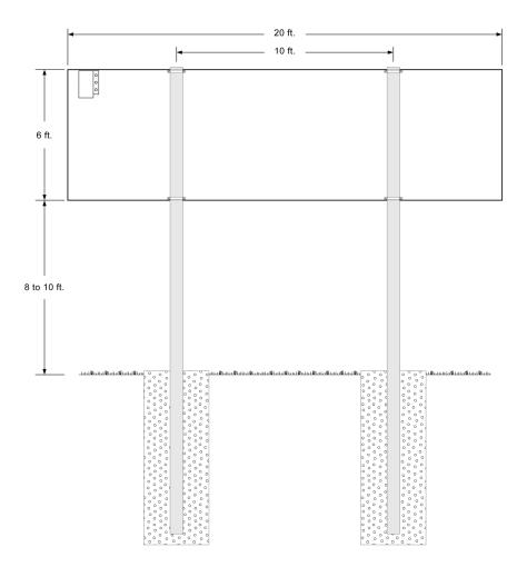
Once you have verified the positions of the posts and the size of the footings, you are ready to dig your holes, pour your concrete, and set your posts. There are several techniques for ensuring proper alignment of the posts. Typically installers will construct a temporary wooden support frame to hold each post in place while the concrete sets. Having plumb posts in the proper position is the key to a smooth mechanical installation.
