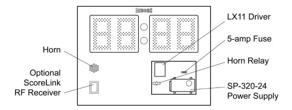
If your scoreboard system includes a ScoreLink wireless data kit, the receiver unit will be in the lower left corner of the display face, and the internal Horn will be mounted just above that spot.
