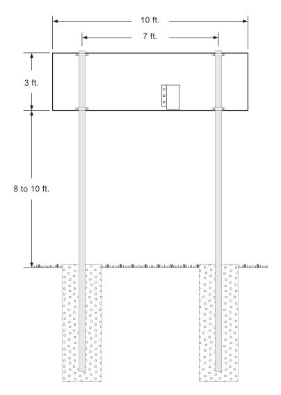
Once you have verified the positions of the posts and the size of the footings, you are ready to dig your holes, pour your concrete, and set your posts. There are several techniques for ensuring proper alignment of the posts. Typically installers will construct a temporary wooden support frame to hold each post in place while the concrete sets. Having plumb posts in the proper position is the key to a smooth mechanical installation.
