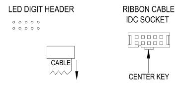
CENTER KEY ON RIBBON CABLE IDC SOCKET MUST POINT IN THE SAME DIRECTION AS THE ARROW ON THE REAR OF THE LED DIGIT.
