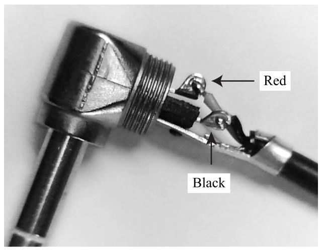
Right-Angle Stereo Plug Wiring Illustration
