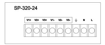
Mean Well #1 Power Supply TerminalsFunctionLine (L)Main AC PowerNeutral (N)Main AC PowerGroundV1 Positive (V1+)V1 Negative (V1-)LX17 DriverV2 Positive (V2+)LX4 DriverV2 Negative (V2-)LX4 DriverV3 Positive (V3+)ScoreLink RF System (if used)V3 Negative (V3-)ScoreLink RF System (if used)
