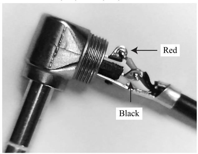
Right-Angle Stereo Plug Wiring Illustration
