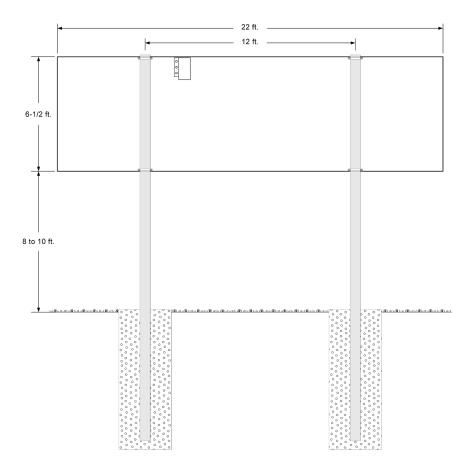
Once you have verified the positions of the posts and the size of the footings, you are ready to dig your holes, pour your concrete, and set your posts. There are several techniques for ensuring proper alignment of the posts. Typically installers will construct a temporary wooden support frame to hold each post in place while the concrete sets. Having plumb posts in the proper position is the key to a smooth mechanical installation.
